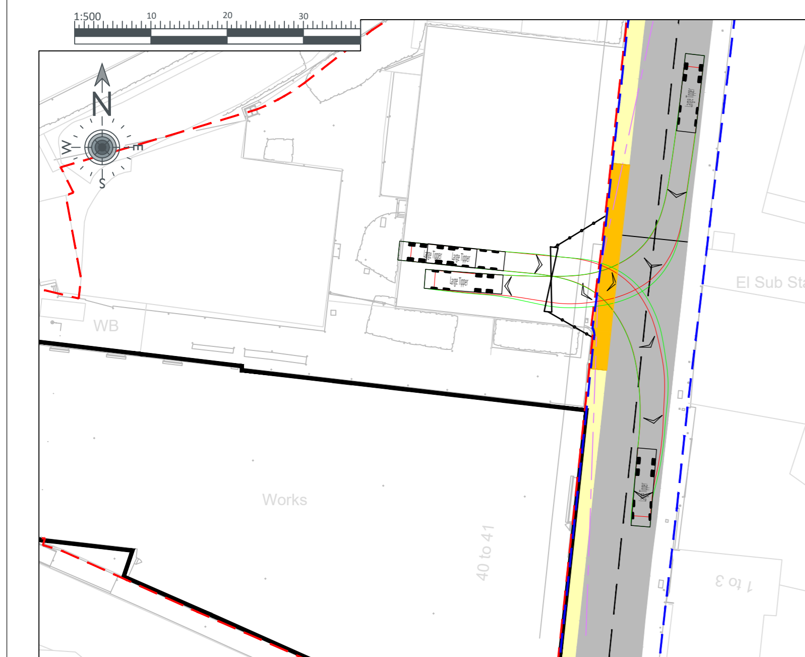
Large Tipper entering and leaving site via right turn at 10mph (1:500)
